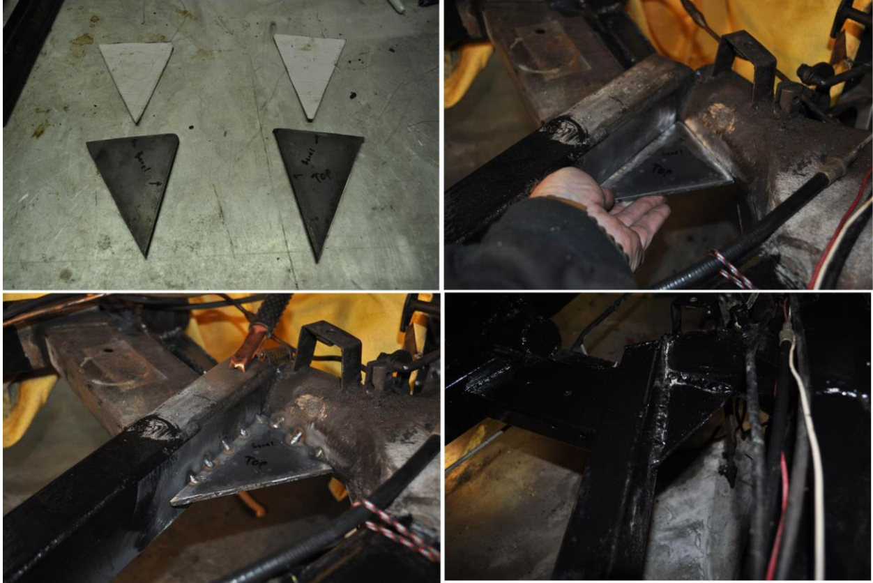
Upper left: gussets cut using cardboard templates, Upper Right: fitting the gusset, Lower Left, the gusset tack welded in place, Lower Right: the complete gusset after the frame is painted.
