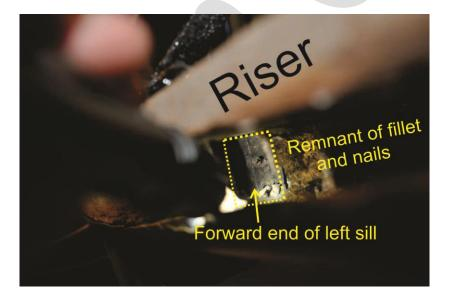
While I had the car up on stands with the floor removed I stripped the metal frame of the car with a pneumatic needle scaler to remove grease, rust and old paint and repainted it with POR 15 paint. I cleaned and sanded the wooden riser and rocker on the exposed sides so they could better absorb CPES. From Keith's drawings, I traced paper cutouts of the sill and rocker for each side. I then taped the cutouts to the door riser to visualize where they were located.
